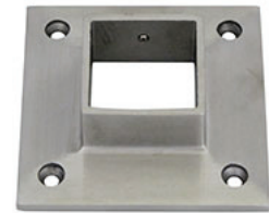
SS108 Square Wall Flange Base 304 Stainless Steel Tube Size: 40x40x2mm Satin Polish Finish
